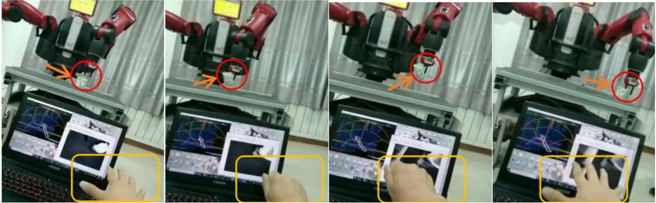
Figure 9: Pick and place based on Leap Motion Controller.
